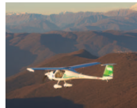
GRIMY SKIES The plane's particle sensor includes an intake tube under the wing that slows air down so that it can be measured. The device picked up high particle levels over the Gulf of Thailand [left].
