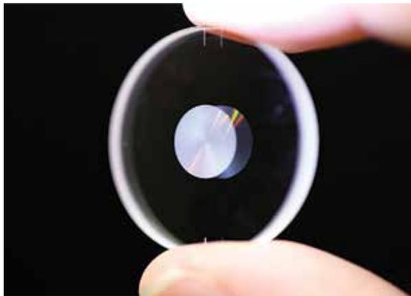
**DISC OF DESTINY:** Using alterations in the way quartz refracts light, we could store data in a superdense form for centuries.
