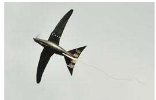
RoboSwift can sweep its wings back for better turning.
