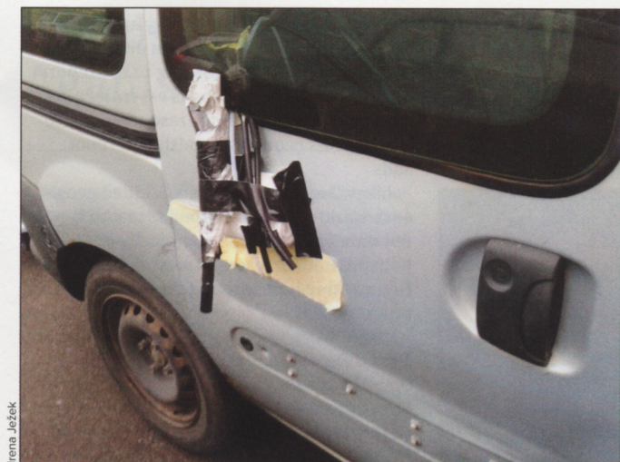
Air intake tubes dangle from a side window of an instrument-laden minivan that researchers used to chase vehicles on Slovenian roads while measuring their tailpipe emissions. The tubes fed exhaust gases into separate instruments for measuring black carbon, nitrogen oxide, carbon dioxide, and particulates.
